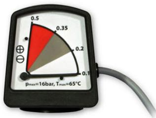
**Differential pressure gauges FAD01C with potential free alarm contact** allow to hook up the differential pressure control of the pre- and after-filter to the common alarm message of each dryer. In order to avoid a false error report due to start-up conditions or short-time peaks, an alarm delay can be set in the dryer control unit. The alarm message then will just be generated, if a too high differential pressure was indicated during the entire delay time interval.
