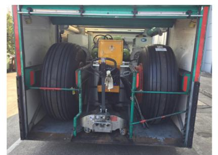
Undercarriage jack along with wheels and tyres ready to fit on an A320 main landing gear, with top up from the internal nitrogen pack using Parker generated gas!
