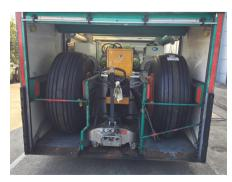
Undercarriage jack along with wheels and tyres ready to fit on an A320 main landing gear, with top up from the internal nitrogen pack using Parker generated gas!
