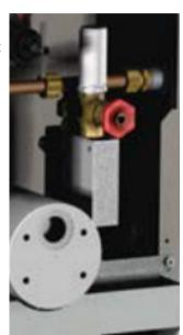
The off-gas by-pass incorporated into the outlet valve block with vent silencer
