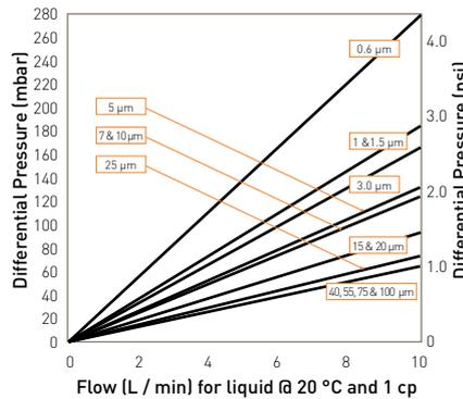
For A size for a given flow rate divide B size differential pressure by 2
