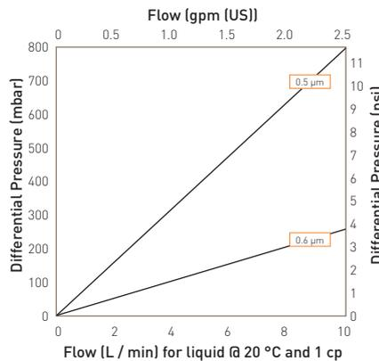
For A size for a given flow rate divide B size differential pressure by 2
