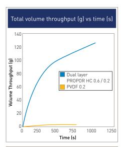
Initial filterability trials on discs: Improvement over incumbent competitor PVDF sterile filter.
