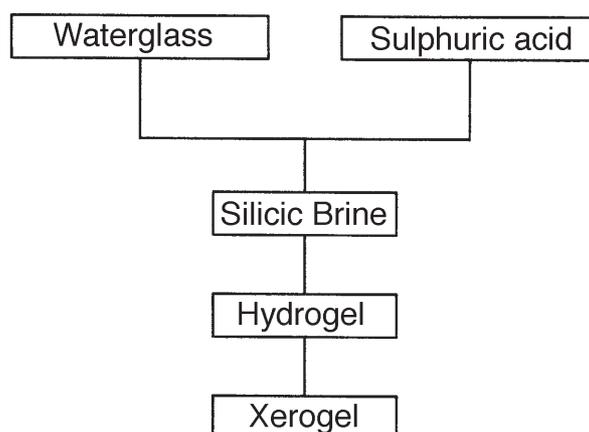
After washing out the sodium sulphate formed in the course of the reaction, the syneric (expelled) water is driven out of the pores by subjection to heat. The hydrogel becomes activated silica gel, xerogel.
