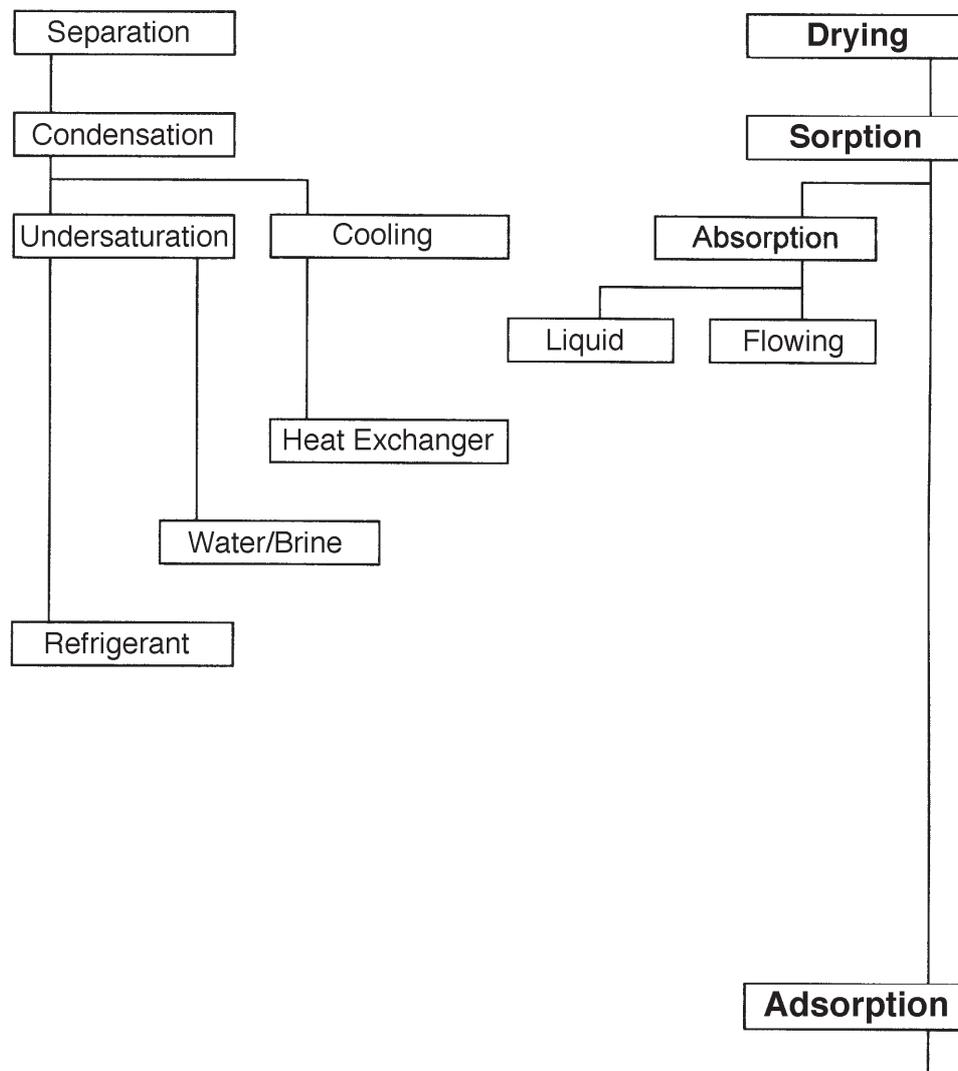
Compressed air dryers operating on the principle of adsorption can achieve pressure dewpoints below 0°C. Compressed air drying by adsorption for pressure dewpoints down to -110°C (state of the art) differ according to the mode of regeneration:
