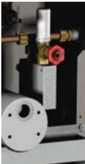
The off-gas by-pass incorporated into the outlet valve block with vent silencer
