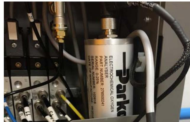
Parker NITROSource's integral oxygen analyser (fitted as standard) measures output gas purity as per the EIGA recommendations. Additionally, 4-20mA outputs or the MODBUS connection allow for remote oxygen indication and data logging, providing complete traceability.
