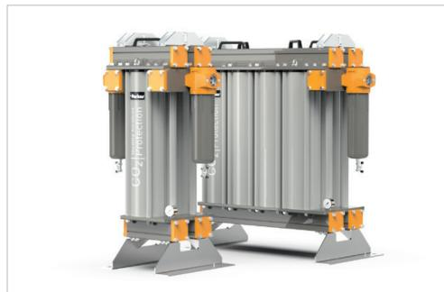
Every Parker model is supplied with integrated filtration as standard. Stage 1 and stage 5 is provided at both the inlet and outlet points of the system. Pre filtration ensures protection of the adsorbent beds from Non-Volatile Organic Residue (NVOR) that may be present in the gas supply and other contaminants down to 0.01 micron. Post filtration ensures no carry- over of particles from the adsorbent beds to 0.01 micron particle filtration.
